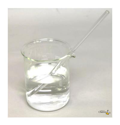
A beaker is used e.g. to collect and mix liquids. Likewise, it can be helpful when preparing solutions as the content can easily be stirred with a glass rod or a stirring bar due to the large opening.
