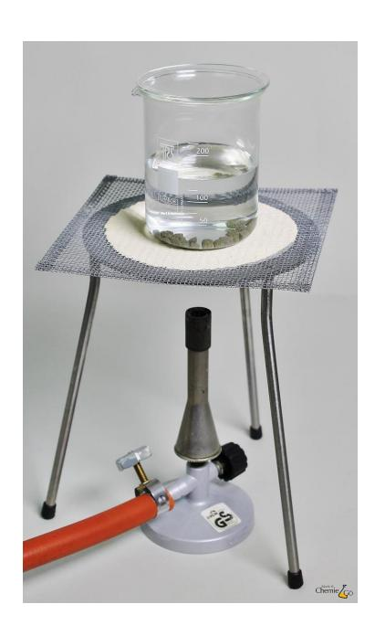
Most beakers are made of borosilicate glass, which makes them resistant to heat and most chemicals.
