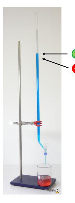
Furthermore, it is important to make sure that one's eye level is on the height of the fluid level when reading it off to guarantee a horizontal and correct read.
