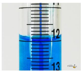
It is decisive to accurately read off the volume of the analytical solution during the titration.
