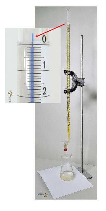
In order to fill a burette with the analytical solution, the valve must first be closed.
