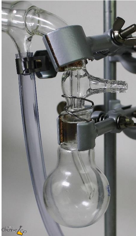
Round-bottomed flask Distillation under normal pressure
