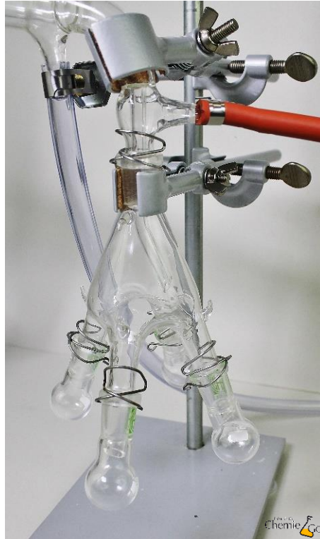
Distillation spider Vacuum distillation
