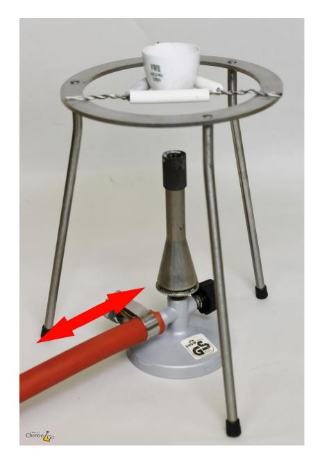
When placing the burner under the tripod, make sure that it can be moved easily if necessary.
