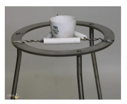
When using a crucible the wire gauze is replaced by a clay triangle. The crucible is placed tightly in the triangle.
