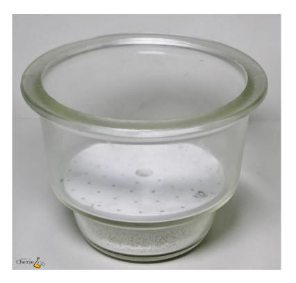
The desiccant is stored in the reservoir below the sievelike platform.
