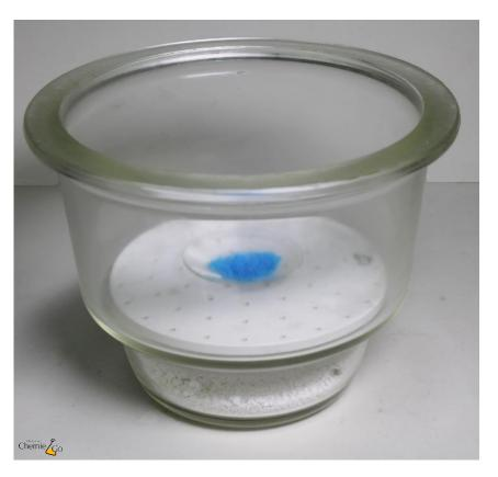
The sample is stored on a watch glass or petri dish, sealed with punctured aluminum foil and placed on the platform.
