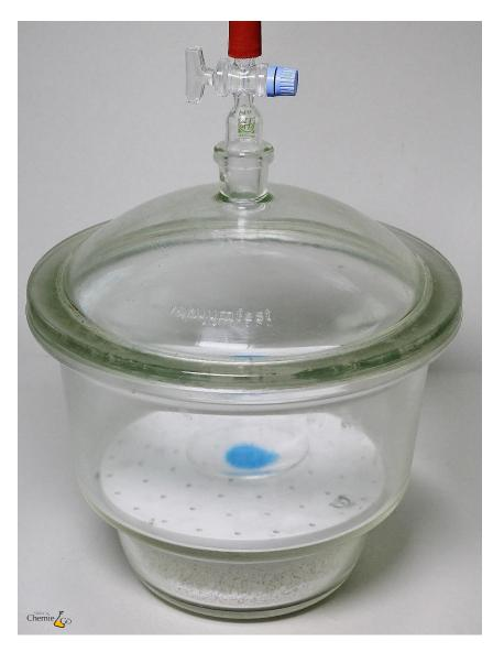
To evacuate the desiccator a hose of a vacuum pump is applied to the stopcock. The hose does not need to be fixed with a clamp.
