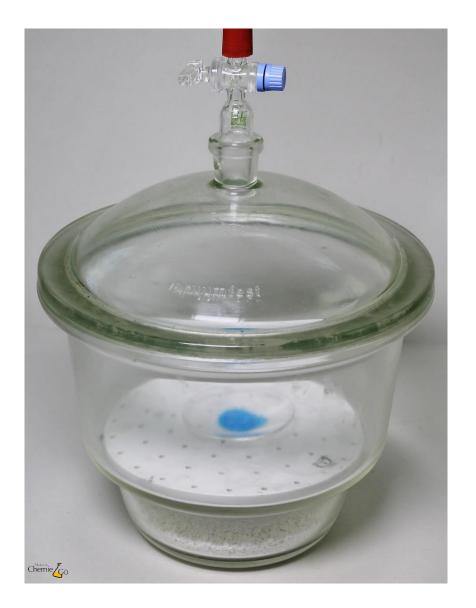
After applying the vacuum the Stopcock is closed and the hose can be disconnected.
