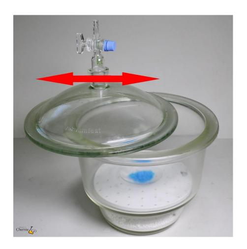
In order to prevent damage the lid should be carefully slid on and off the base. To maintain a good seal, vacuum grease needs to be applied to the flanges.
