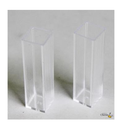
A cuvette is a sample vial for spectroscopic applications, made mostly of plastic or quartz glass.
