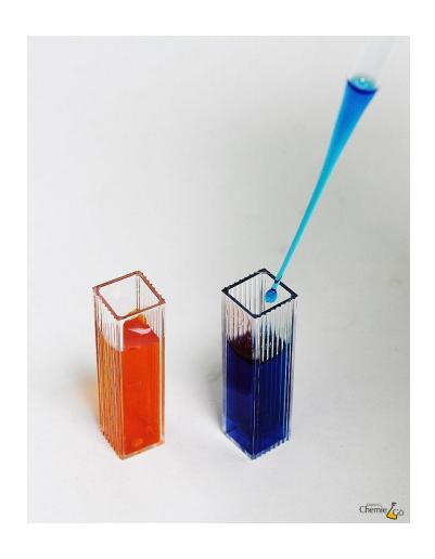
The cuvette is filled with a solution and subsequently placed in the spectrometer.
