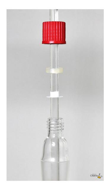
First, the PTFE disk is slid on, which is resistent to chemicals.
