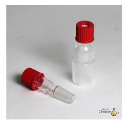
A quick-fit is a ground joint with a screw adapter.
