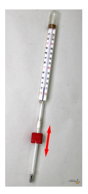
The screw cap with rubber gasket and PTFE-disk is slid on the thermometer.
