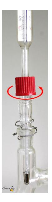
The glass adapter is secured with a clip and the thermometer with screw cap is screwed on the quick-fit.
