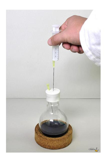
Using a canula, the septum can be pierced and substance removed. When doing this, it is important use a second canula for pressure equalization.
