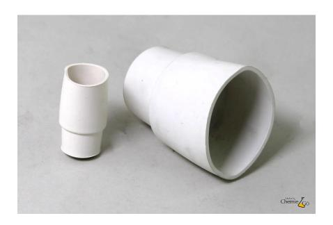
To seal a flask, the septum is first placed on the flask (left) and then flipped over the ground-glass joint (right).
