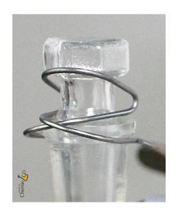
Ground-glass stoppers are used to cap glass apparatuses with ground-glass joints and should be secured with a joint clip.
