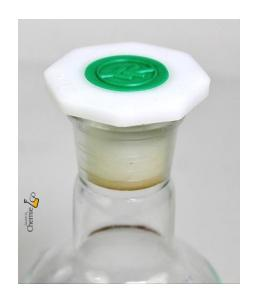
Plastic stoppers are used to cap glass equipment. They can also be used to seal extraction vessels.
