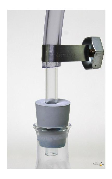
Rubber stoppers can be pierced and used e.g. to secure glass tubes.
