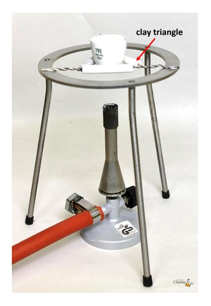
A crucible can be positioned optimally above a gas burner with the help of a clay triangle.
