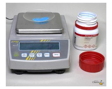
The desired amount of the substance is weighed out and the displayed value is noted down.
