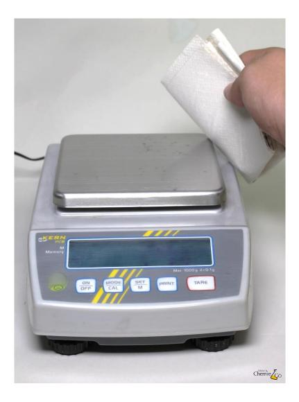
The sample container is removed from the weighing plate and the balance is tared. If necessary, the surface is cleaned with a paper towel.
