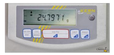
Finally, the difference between the two values is calculated to determine the exact weight of the sample.
