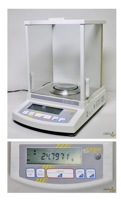
The side window is closed and after some time the weight of the sample container can be noted down.
