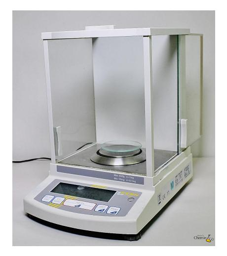
After opening the side window, a sample container (here: watch glass) is placed on the weighing plate.
